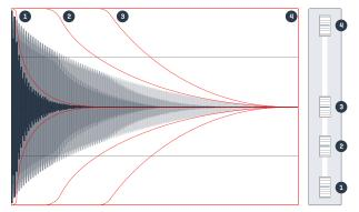
multiplier curve is a dynamic combination of a hold feature (multiplier = 1) and the tail with decreasing factors for longer time frames. This complex relationship is fixed and not editable in its parameters. The illustration above gives an idea, how the **Release** feature shapes the amplitude of a sample in relation to the fader position. Curves shown are optimized for visualization purposes and don't claim to be exact.
