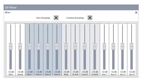
Note, that **Snare Style** and the **Mixer Volume Faders** are parameters stored in the drum kit, whereas fader grouping is stored in the default device data bank. A detailed description of drum kit parameters is topic of the **Kit Editor** mode (see section 9.2.1.5 Drum Kit Presets - Parameters on page 44).
