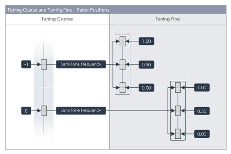
With the illustration in mind, the best practice for changing the pitch of the sound samples is consequently blocking out the rough pitch region with **Tuning Coarse** and fine tune it afterwards with the help of **Tuning Fine**.
