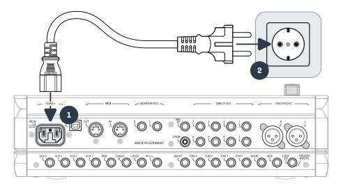
With the cord connected correctly the **[Power]** button lights up in red. The device is in standby mode and ready to be explored. Press the **[Power]** button to boot the apparatus.
